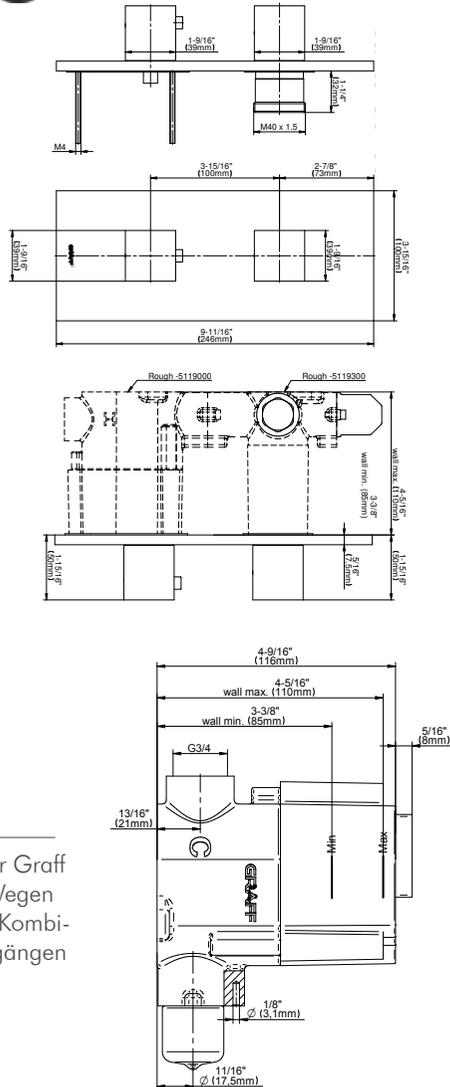
**UNTERPUTZ-EINBAUKÖRPER 3/4" THERMOSTAT**
